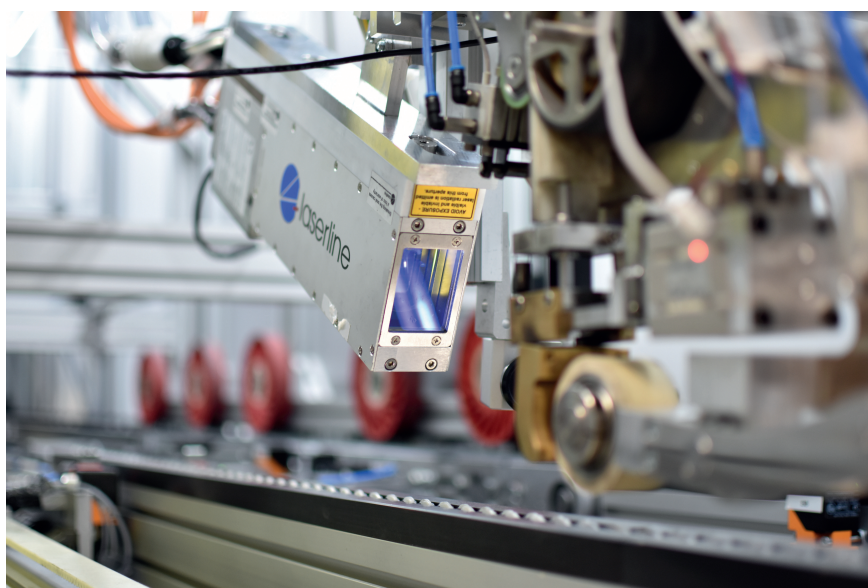
The direct diode laser LDMdirect from Laserline facilitates installation in assembly lines thanks to its small housing width of only 50mm. Another plus point: Several processing heads can be integrated into one mounting © AZL Aachen GmbH
